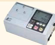
For indoor air quality measurement in buildings and classrooms. Auto sensitivity calibration by suctioning standard gas after setting the value. High stability for continuous measurement.
