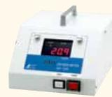
For measurement of residual Oxygen in inert gas. Compact design with a built-in suction pump.
